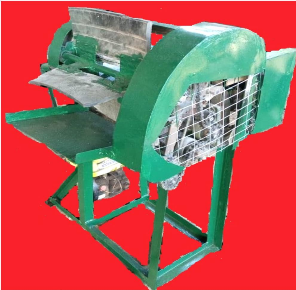
Figure 1.0: A fabricated coconut dehusking machine
